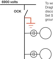
To work on MG Sets or DC Motors on a Dragline or Shovel, open and lock the visible disconnect that removes power from the MG Set Stator or Drive isolation Transformer then ground the load side of the switch.
